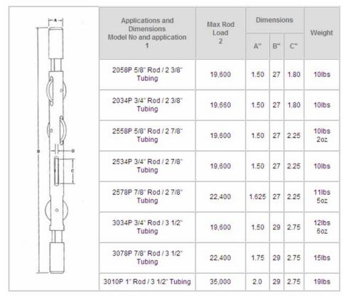
Figure 13: Wheeled rod guides for rod protection in deviated wells.
