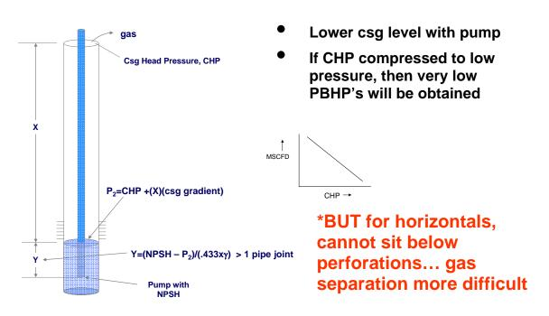
Figure 3. How pumps dewater in a near vertical well.
