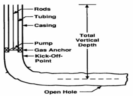
Figure 4: Showing pump can be set in the near vertical section of a horizontal well.
