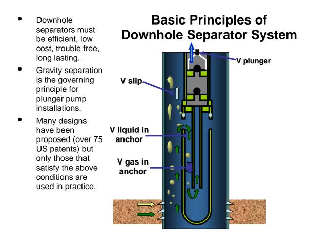
Figure 5: Review of what gravity segregation gas separator or "poor boy" gas separator is. From Echometer.
