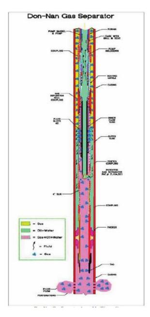
Figure 10: Improved packer separator with increased radial symmetry and other features.
