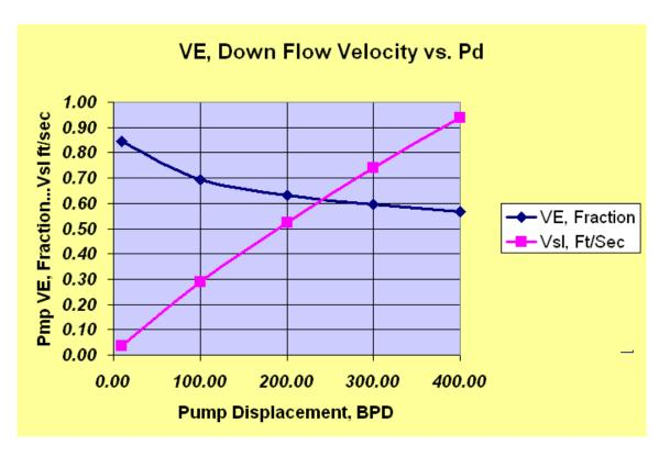
Figure 8: Showing separator performance can be continuous relationship that is function of GOR, pressure, downflow area and fluid properties. However the best performance will still be with the downflow velocity below  $\frac{1}{2}$  ft/sec.
