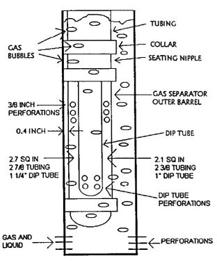
Fig. 3 Conventional Separator Above Formation
