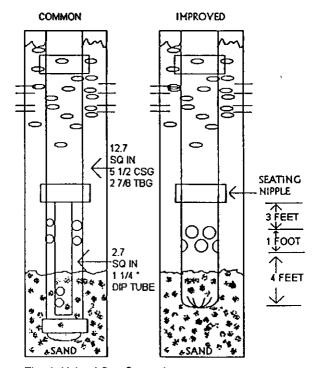
Fig. 1 Natural Gas Separators
