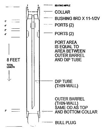
Fig. 4 COLLAR-SIZE GAS SEPARATOR DETAIL
