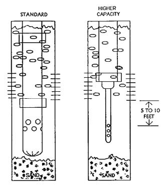
Fig. 2 Higher Capacity Natural Gas separator
