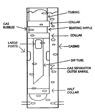
Fig. 5 Collar-Size Gas Separator in Casing
