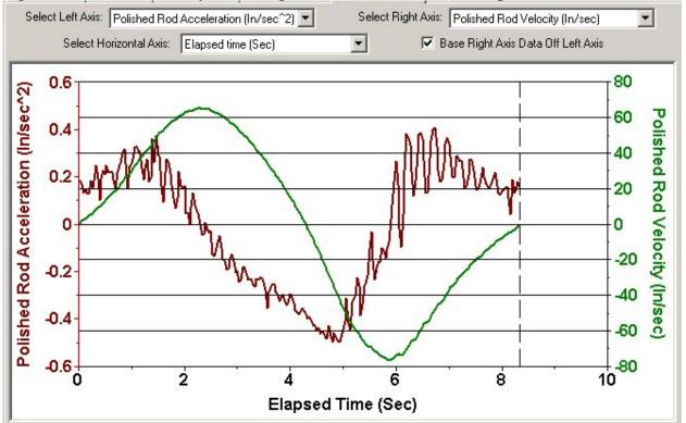
Fig. 1 – Polished Rod Velocity is the Integration of Acceleration with Respect to Time.
