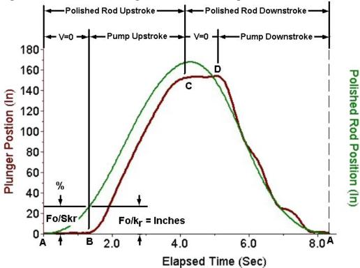
Fig. 4 – Polished Rod and Plunger Position Versus Elapsed Time for Anchored Tubing.
