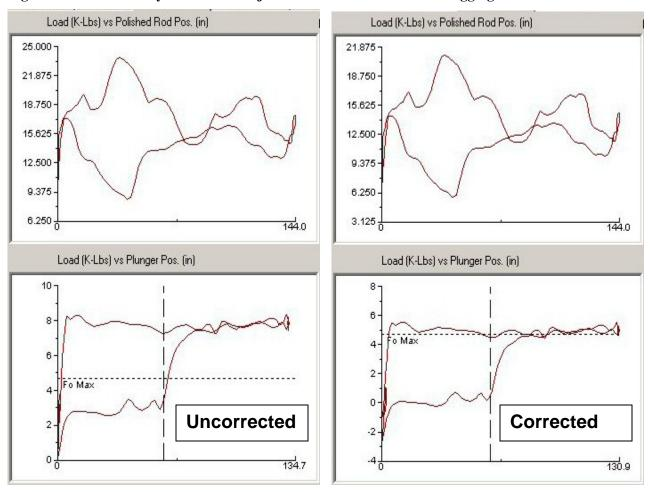
Fig. 8 – Surface PRT Dynamometer Adjusted for Load Offset due to Tagging on the Down Stroke
