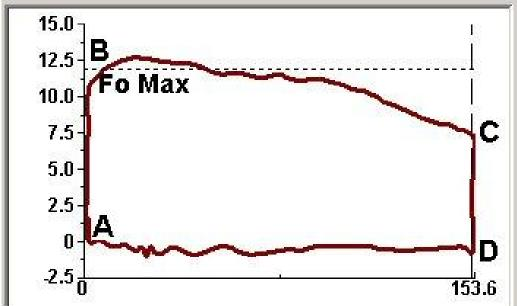
Fig. 6 – Example Pump Card w/ Load (k-lbs) and Position (inches)
