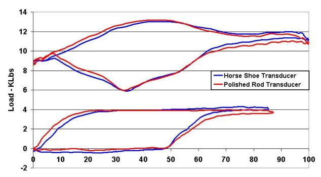
Fig. 9 – Comparison of Polished Rod and Pump Dynamometer Cards for PRT and Load Cells
