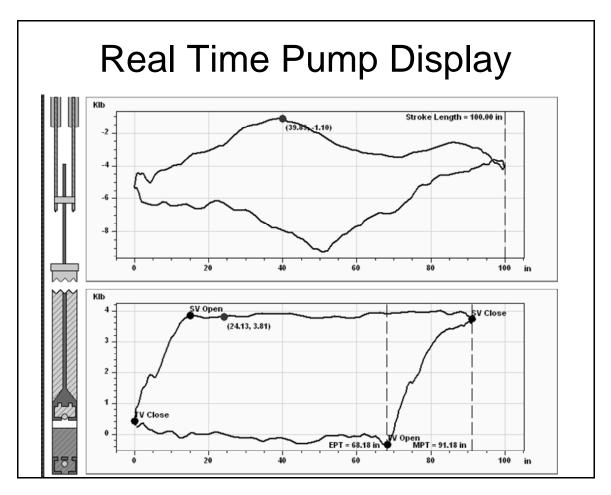
Figure 14 – Detail of Real-time visualization of pump operation with coordinated display of polished rod travel and loading.
