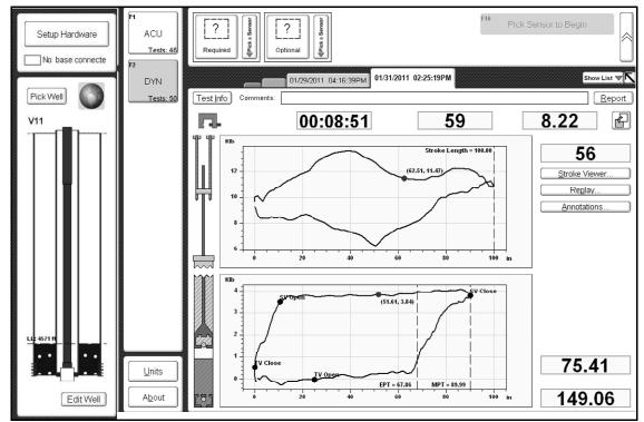
Figure 9 - Real-time Presentation of Surface and Pump Dynamometer Recording Coordinated with Fluid Level Measurement and Visualization of Fluid Distribution in Wellbore.
