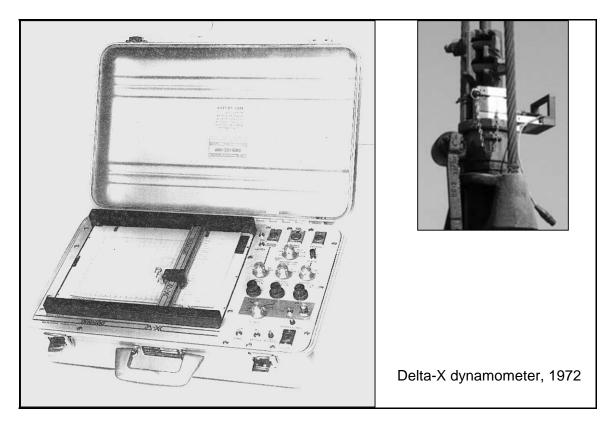
Figure 4 – Portable Electronic Recording of Dynamometer Data.(Delta-X)
