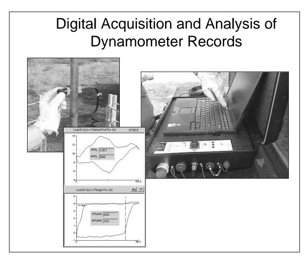
Figure 7 – State of the art dynamometer data acquisition and processing system
