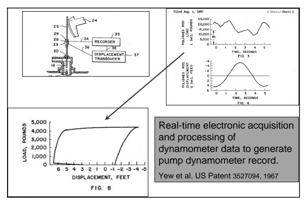
Figure 6 – Real-Time electronic calculation of pump dynamometer card.
