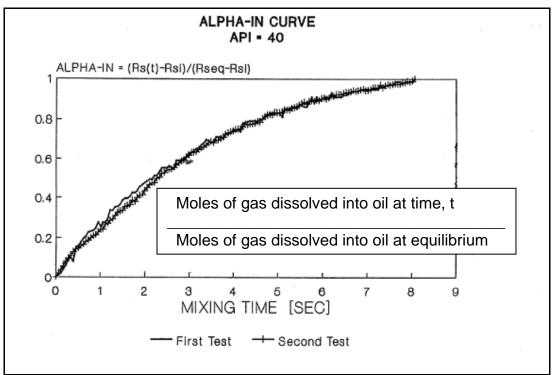
Figure 10 – Dimensionless rate of gas dissolution as a function of time. Ref 8.
