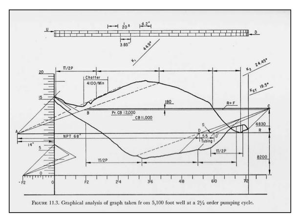
Figure 3 – Graphical Analysis of Surface Dynamometer Record,, (Slonneger 1961)
