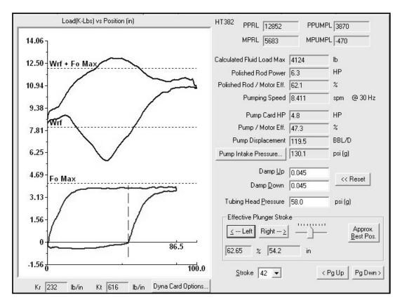
Figure 8 – Detailed analysis of dynamometer data for one pump stroke.
