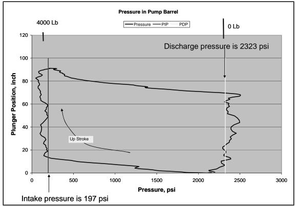
Figure 13 – Pressure Variation inside Pump Barrel during one Plunger Stroke
