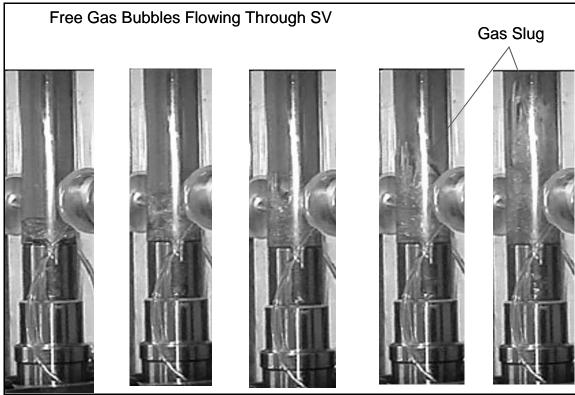
Figure 12 – Agitation and turbulence for two-phase flow through standing Valve. (Ref.9)
