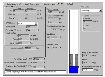
build-up measurement allows calculation of the casing annulus gas flow rate and the gradient of the gaseous liquid column if free gas is bubbling up through the liquid. Software calculates the producing bottomhole pressure, maximum production rates, pump intake pressure, casing annulus gas flow rate and other parameters. This single-shot acoustic liquid level depth test is displayed as shown so the operator can visualize and understand the performance of the well.
