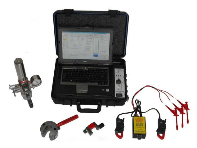
THE WELL ANALYZER IS A PORTABLE COMPUTERIZED INSTRUMENT FOR OBTAINING A COMPLETE WELL ANALYSIS
