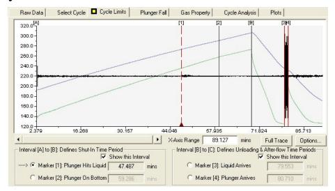
by determining the position and velocity of the plunger throughout the cycle and calculating gas and liquid flow rates into and out of the wellbore as a function of the measured pressures.
