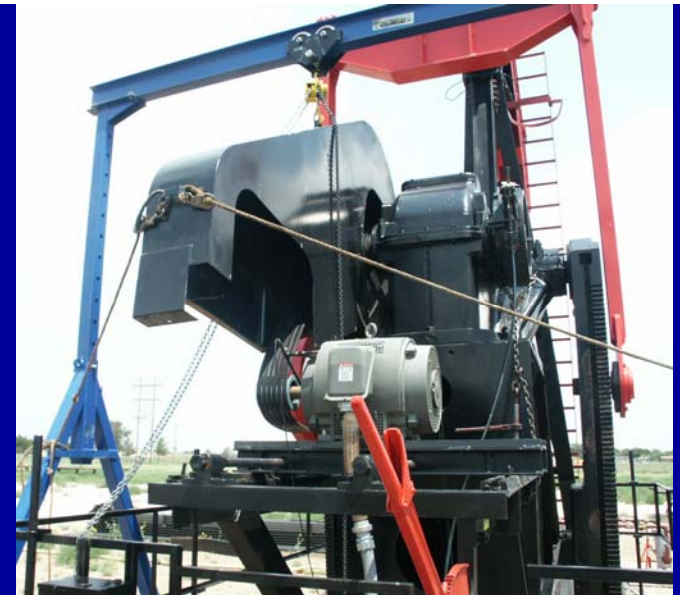
Used Gantry Crane to Lift Belt Guard Quick Sheave Change ~ 2 hours
