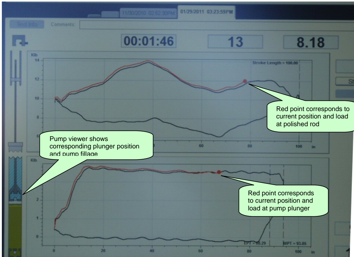
Figure 5 – Real Time Visualization of Pump Fillage and Dynamometers for stroke 13 (red dot and line). Black lines show dynamometer record for the preceding stroke number 12.
