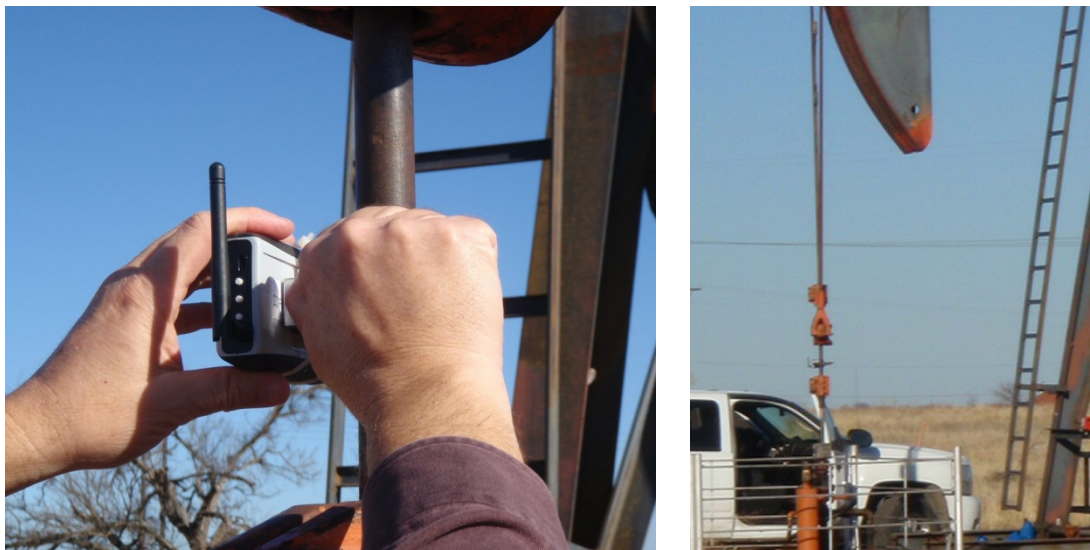
Figure 2 – Wireless Polished Rod Transducer (WPRT) Installation
